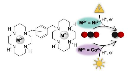
Figure 1. General structure and idea of the application of bimetallic cyclam complexes for the electrochemical and photochemical CO<sub>2</sub> reduction.
